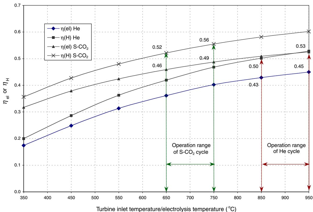
FIGURE G-5 Power cycle net efficiency ( $\eta_{\text{el}}$ ) and thermal-to-hydrogen efficiency ( $\eta_{\text{H}}$ ) for the gas turbine modular helium reactor (He) high-temperature electrolysis of steam (HTES) and the supercritical CO<sub>2</sub> (S-CO<sub>2</sub>) advanced gas-cooled reactor HTES technologies. SOURCE: Yildiz and Kazimi (2003).
