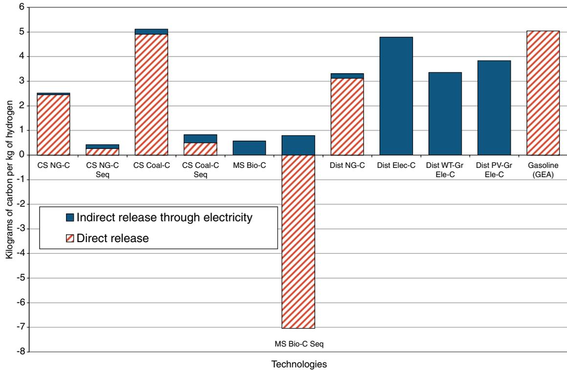
FIGURE 5-9 Estimates of unit atmospheric carbon release per kilogram of hydrogen produced by 10 current hydrogen supply technologies. See Table 5-2 and discussion in text. NOTE: GEA = gasoline efficiency adjusted.
