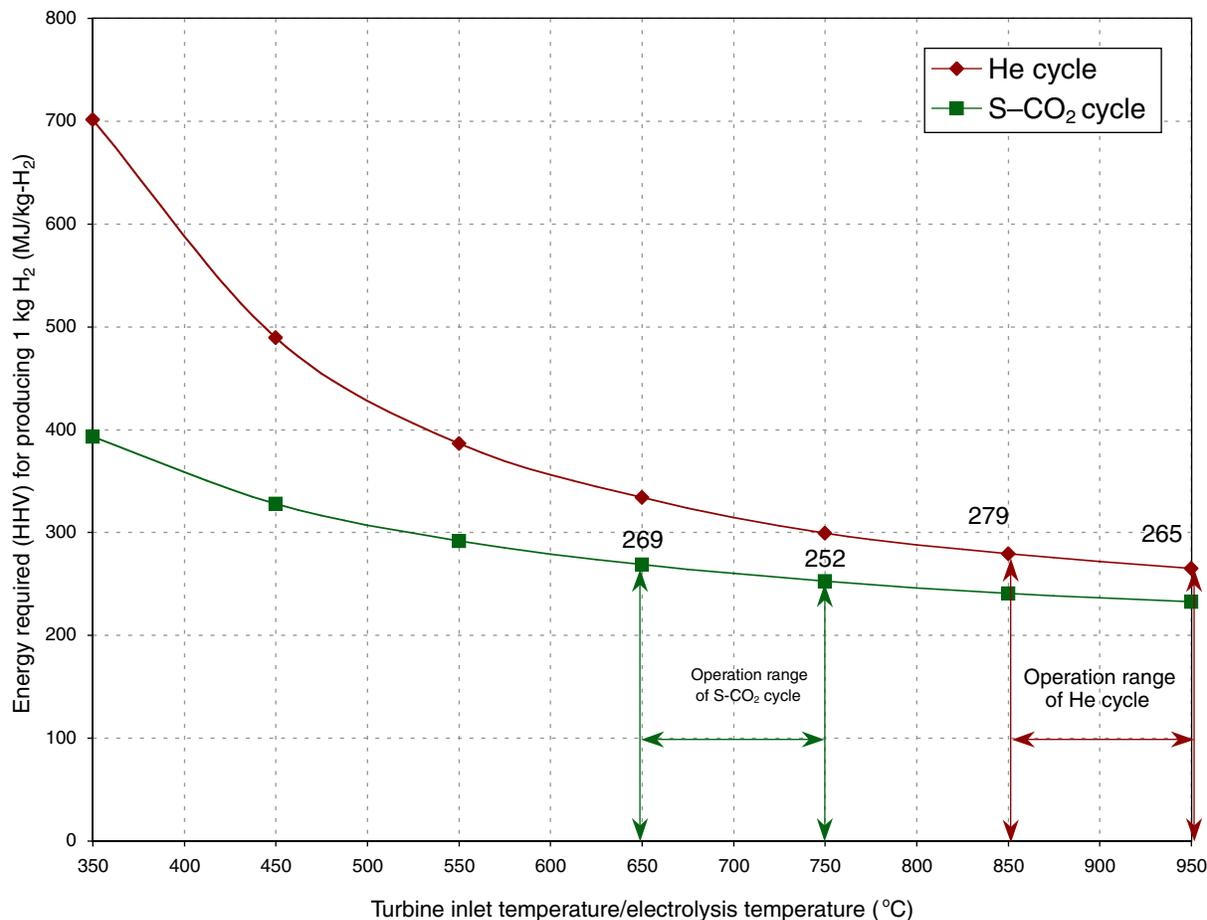
FIGURE G-6 The energy needs for hydrogen production by the gas turbine modular helium reactor (He cycle) high-temperature electrolysis of steam (HTES) and the supercritical CO<sub>2</sub> (S-CO<sub>2</sub> cycle) advanced gas-cooled reactor HTES technologies. NOTE: HHV = higher heating value.
