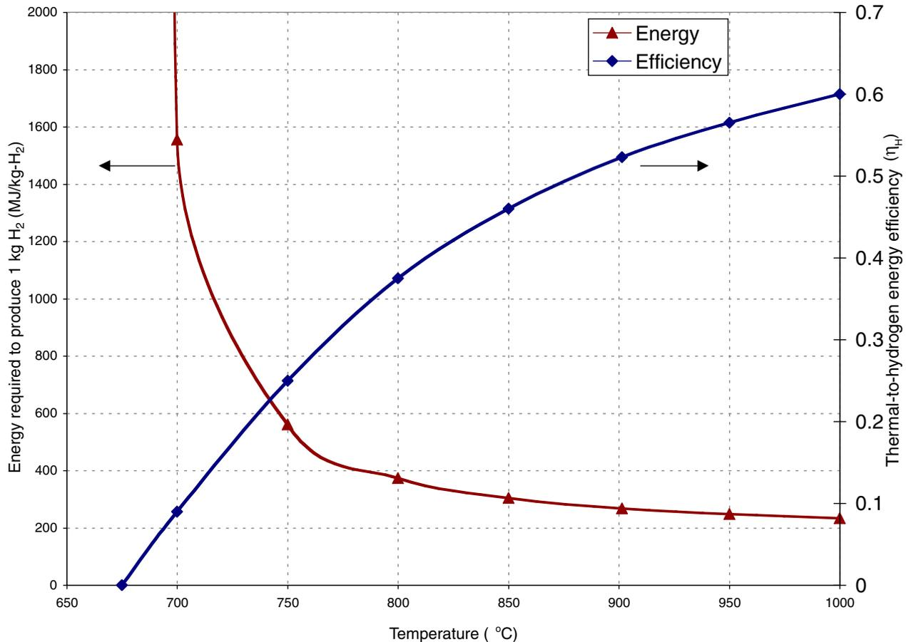
FIGURE G-8 Estimated thermal-to-hydrogen efficiency ( $\eta_H$ ) of the sulfur-iodine (SI) process and thermal energy required to produce a kilogram of hydrogen from the modular high-temperature reactor-SI technology. SOURCE: Brown et al. (2003).
